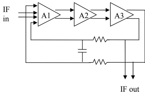
**Fig. 4. Block diagram of SDLVA dc feedback offset error compensation.**
