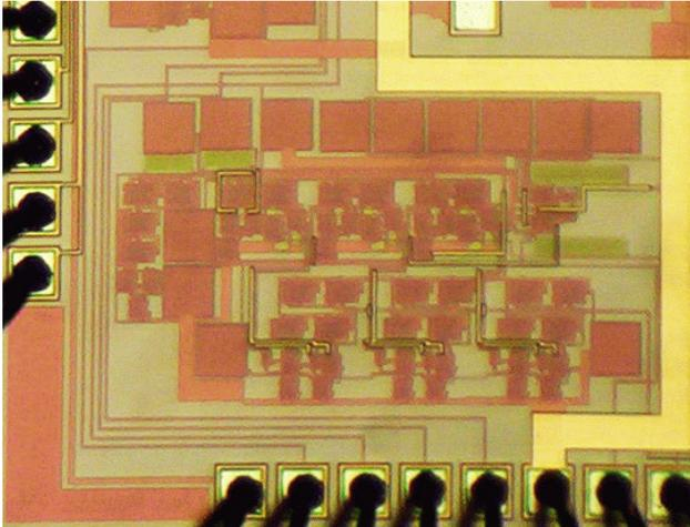
**Fig.5** Photograph of SDLVA fabricated in 0.5 micron CMOS.
