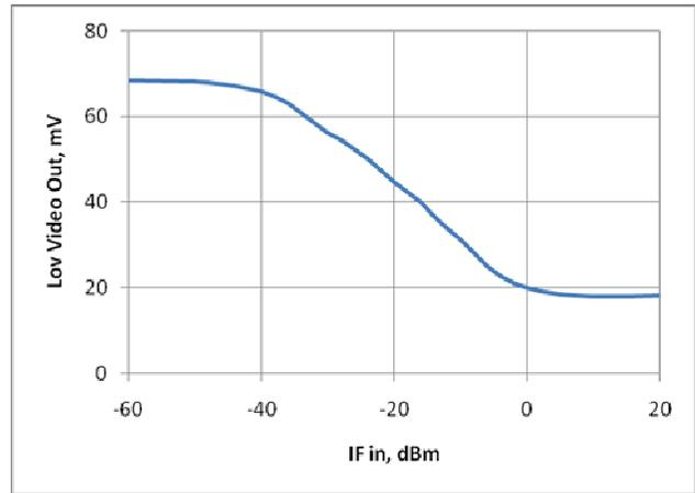
**Fig. 6.** SDLVA measured response for a 1 MHz input signal. Horizontal axis is IF input signal strength in dBm, vertical axis is measured log detected video output voltage.
