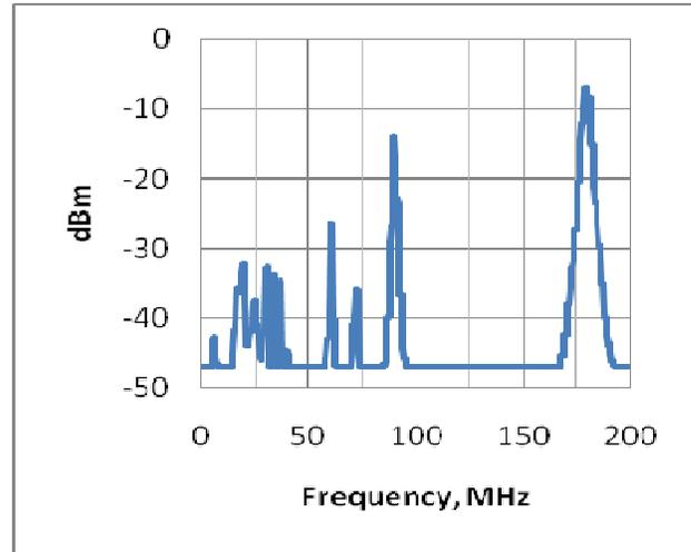
**Fig. 9. Spectrum analyzer: measured spectrum of 180 MHz -10 dBm sinusoid. Horizontal axis is RF input frequency, vertical axis is logarithmic video output converted to equivalent power level in dBm.**
