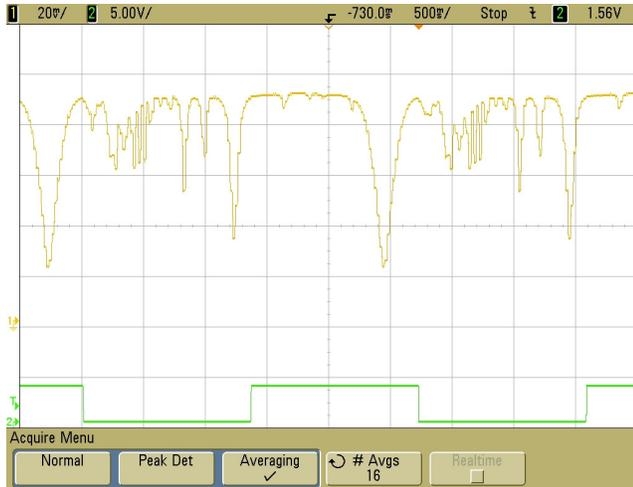
**Fig. 8. Spectrum analyzer: measured spectrum of 180 MHz -10 dBm sinusoid. The Horizontal axis is RF input frequency, from 0 to 200. Large dip in upper trace indicates strong 180 MHz RF input signal (axis inverted).**
