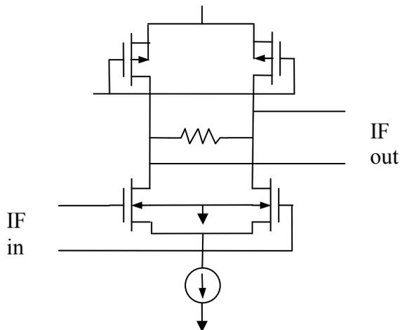
**Fig. 3. Amplifier schematic**
