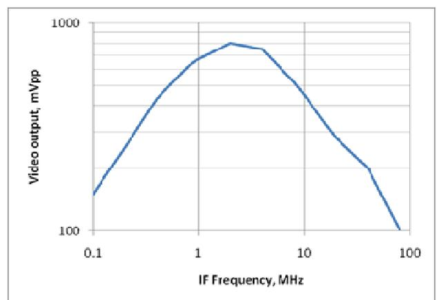
**Fig. 7.** SDLVA measured frequency response for a 1 MHz input signal at 12 mVpp. Horizontal axis is IF input signal frequency in MHz, vertical axis is measured linear video output voltage peak-to-peak.
