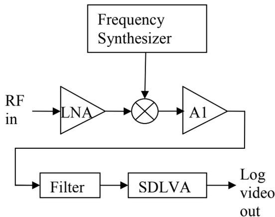
**Fig. 1. Block diagram of frequency-synthesized spectrum analyzer. Spectrum analyzer input is denoted “RF in,” and spectrum analyzer output is denoted “Log video out.”**
