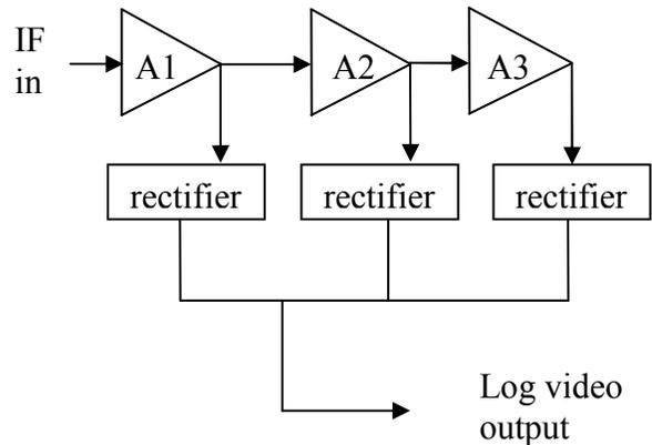
**Fig. 2. Block diagram of SDLVA. SDLVA input is “IF in,” and spectrum analyzer output is “Log video out.”**
